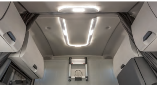
LED Interior Lighting
